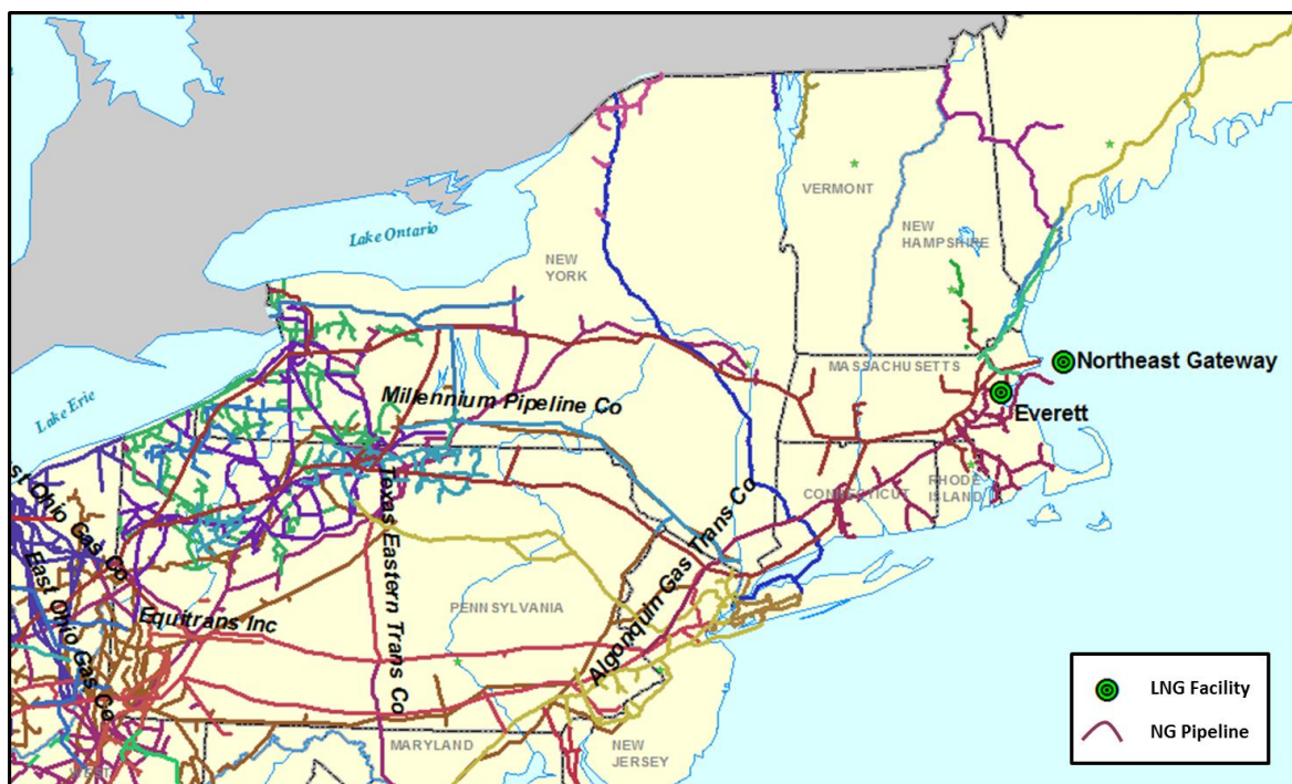
Figure 31: Map of LNG Facilities and Natural Gas Pipelines in the Northeast US 116
